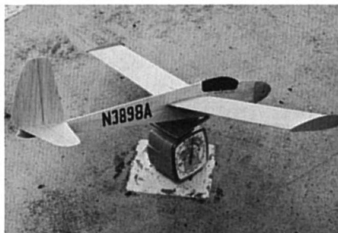
The 36-in. winged glider should weigh under 4 oz. Clay is suitable and easily varied nose weight.
